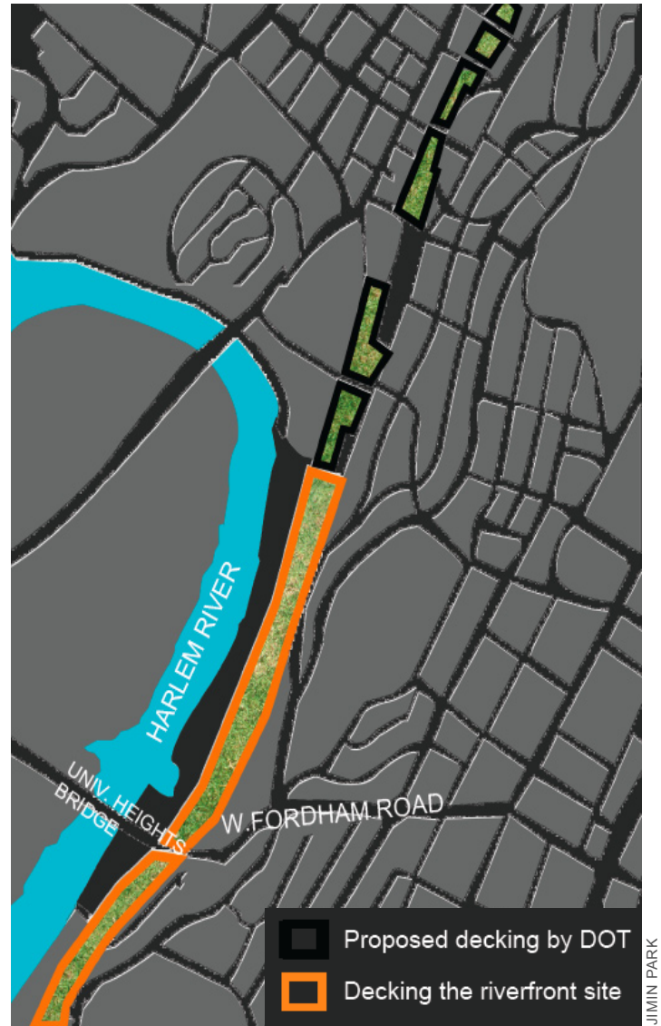
Above: Map showing locations along the Major Deegan where decking is already proposed by DOT (outlined in black), and future potential decking sites over the Expressway along the study site (outlined in orange).
